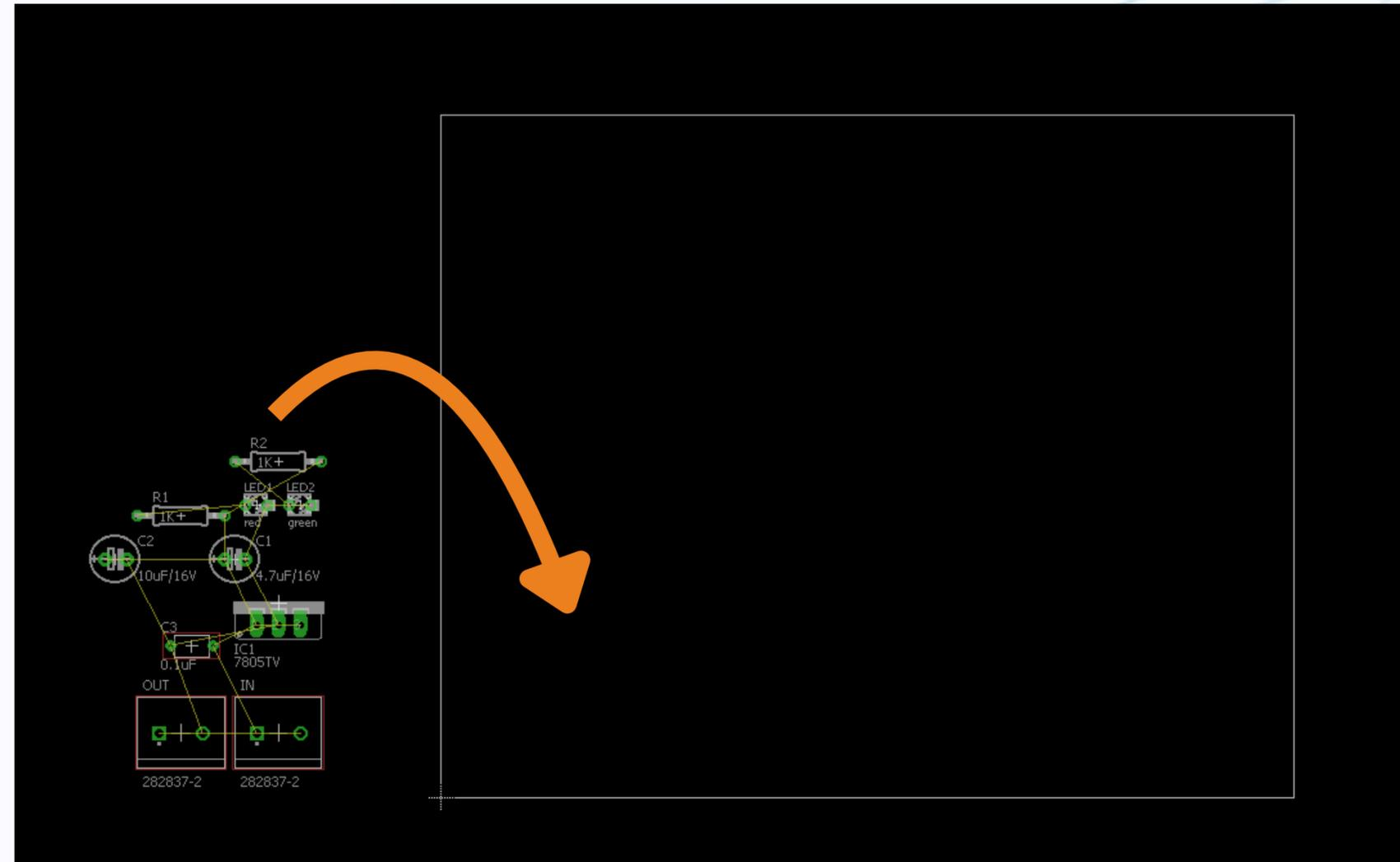
**Arrange the components inside the board layout**
