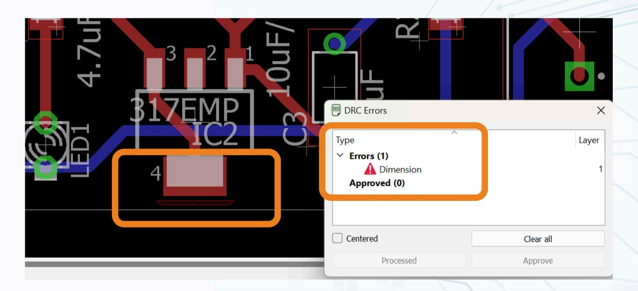
Insufficient gap between border and components
