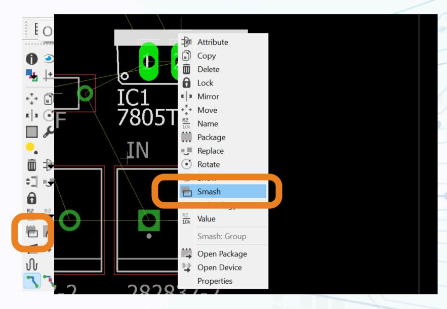
Smash tool to configure the Name & Value of a components
