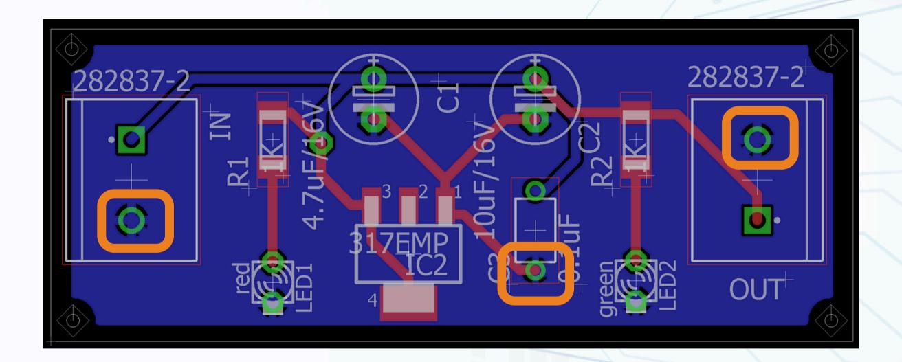
All the GND terminals are connected to the copper pour
